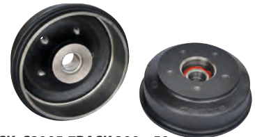
Bremstrommel BPW S2005-5RASK, S2005-7RASK 200 x 50
